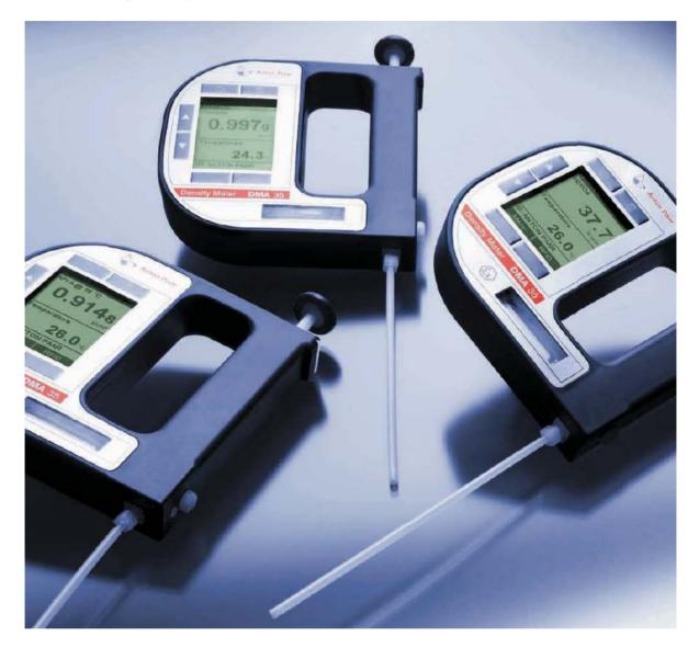
The DMA 35 is the new generation of Anton Paar portable density meters, using the oscillating Utube technology. The sample to be measured is filled into a U-shaped tube which is caused to vibrate. The resonance frequency of the fluid oscillation inside the U-tube is influenced by the mass and therefore by the density of the sample. The advantages of this measuring technique include both good repeatability and high precision.
